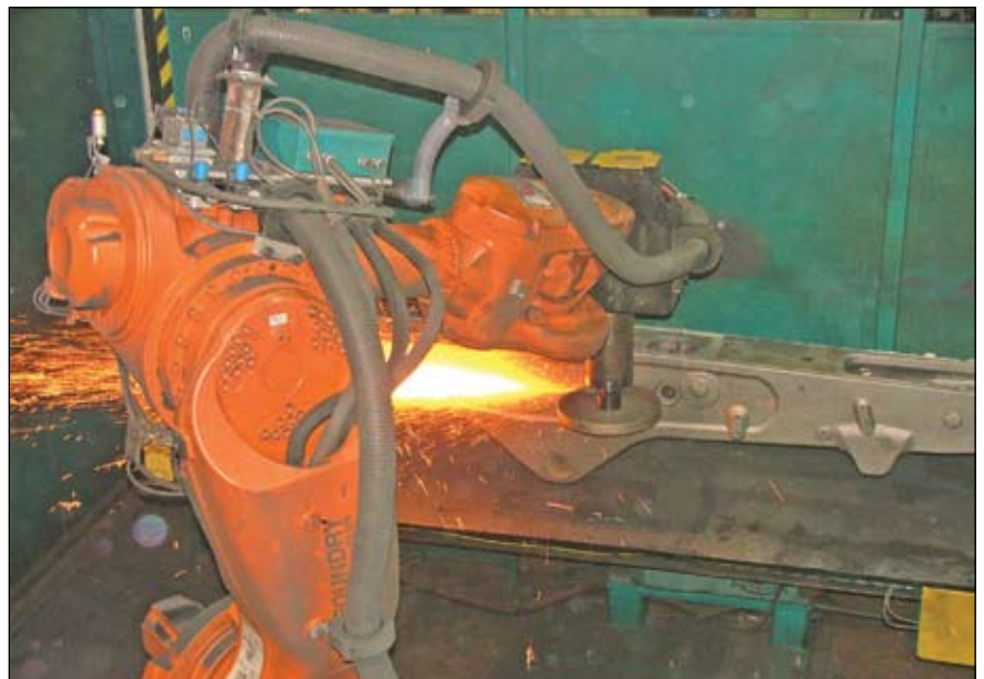
American Castings' new automated grinding cells have reduced grinding time by nearly 60%.
